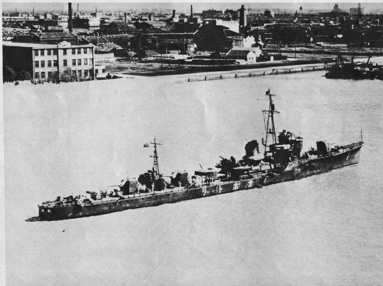
Torpedo boats of the Chidori-Otori Class are used as convoy guards. Light ships, the Chidoris have lean, swift lines. The bridge is low and
